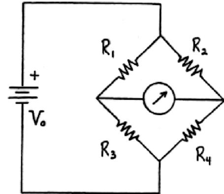
$V_0 =$  Lambda power supply, set to about 4 V. (You can try larger values — up to 40 volts. This will increase your sensitivity for balancing the bridge, but will introduce more heating which will make the resistance values change. So it’s a trade-off. If you want, you can experiment with different values of  $V_0$  when you do part 4.)
