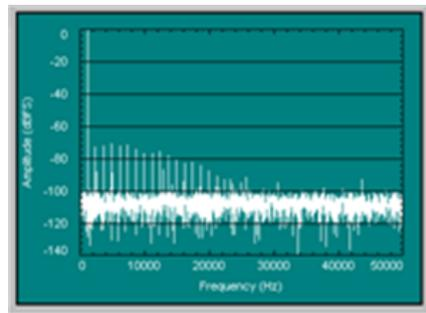
**Figure 1:** An improperly driven, 12-bit SAR ADC can produce unwanted noise and harmonic distortion. In this diagram, the signal-to-noise ratio (SNR) is 69.76 dB full scale, and the total harmonic distortion (THD) is 63.34 dB full scale for a converter that performs at an SNR of 71.82 dB full scale and a THD of 78.82 dB full scale.
